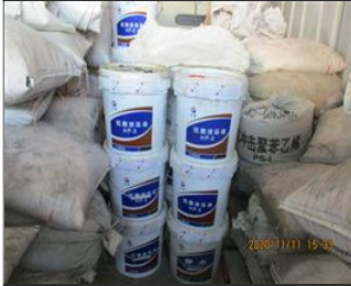
Photo of non-conformity Hydraulic oil not stored in secondary containment and no relevant MSDS posted onsite.JPG
