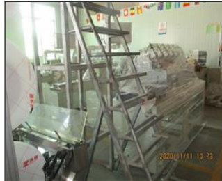
Photo of non-conformity No handrail for staircase.JPG
